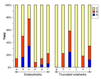
**Fig. 3.** Yield measured in self-folding experiments on nets with varying  $V_c$  and  $R_g$ . (*A–F*) Dodecahedral nets in the order  $V_c=2$ , 6, and 10, and  $R_g=1,102.2$ , 800.9, and 693.7 μm, respectively. (*G–L*) Truncated octahedral nets in the order  $V_c=2$ , 7, and 12, and  $R_g=1,306.3$ , 912.7, and 795.0 μm, respectively.
