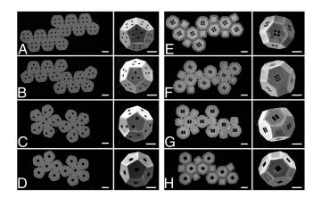
**Fig. 4.** Self-folding experiments on high  $V_c$  nets with varying  $R_g$ . Optical and SEM images. (A–D) Dodecahedral nets with  $V_c$  = 10 and  $R_g$  = 810.2, 797.4, 755.4, and 747.7  $\mu$ m, respectively. (E–H) Truncated octahedral nets with  $V_c$  = 12 and  $R_g$  = 911.6, 870.2, 867.4, and 852.8  $\mu$ m, respectively. (Scale bar: 300  $\mu$ m.)
