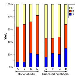
**Fig. 5.** Yield measured in self-folding experiments on high  $V_c$  nets with varying  $R_g$ . (A–D) Dodecahedral nets with  $V_c=10$  and  $R_g=810.2$ , 797.4, 755.4, and 747.7  $\mu$ m, respectively. (*E–H*) Truncated octahedral nets with  $V_c=12$  and  $R_g=911.6$ , 870.2, 867.4, and 852.8  $\mu$ m, respectively.
