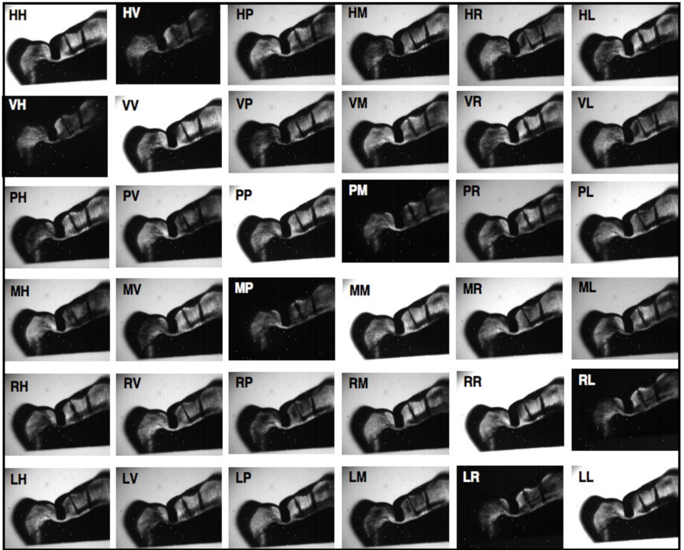
Fig. 3. Unprocessed intensity images of 1 a tooth section (1 mm thick) used to construct the matrix elements of the Mueller Matrix. The notation is as follows: the first term represents the input polarization state while the second term represents the output polarization state for H, V, P, M, R and L.
