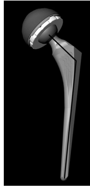
Fig. 2 A computer-generated image shows the hip arthroplasty design. Implant design variables included head size, neck diameter, and neck-shaft angle (thick black line).
