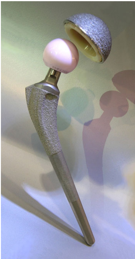
Fig. 1 The MHP femoral component, introduced in 1984, is a double-tapered titanium stem with a proximal porous plasma-sprayed surface applied circumferentially around the stem. The middle section is grit-blasted and the distal section has a matte finish. The device is available in 14 standard offset sizes with a neck angle of 136.5^\circ , diameters from 6 to 19 mm, and lengths from 135 to 180 mm, and 10 lateralized offset sizes with a neck angle of 131.5^\circ , diameters from 8 to 17 mm, and lengths from 145 to 180 mm. (Reproduced with permission of Joint Implant Surgeons, Inc, New Albany, OH.)
