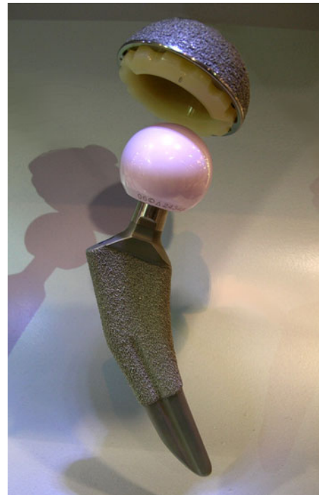
Fig. 2 The TaperLoc ® Microplasty ™ femoral component is a tapered, titanium, porous plasma-sprayed device available with either standard or lateralized offset and in 13 sizes, with diameters ranging from 5 to 25 mm and lengths ranging from 95 to 135 mm. The neck shaft angle is 138^\circ for both standard and lateralized offset options, with lateralization achieved by shifting the trunnion medially. (Reproduced with permission of Joint Implant Surgeons, Inc, New Albany, OH.)
