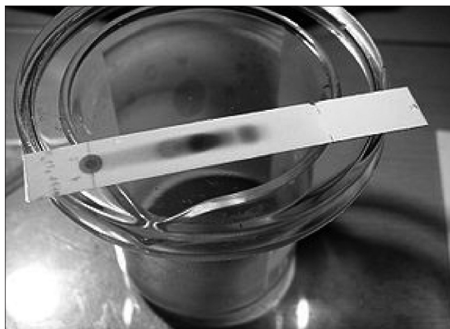
Figure 4: Separation of different chemical constituents by TLC
