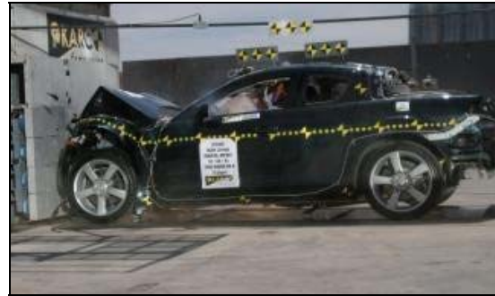
Figure1: NCAP Crash Test into a Rigid Wall Barrier
