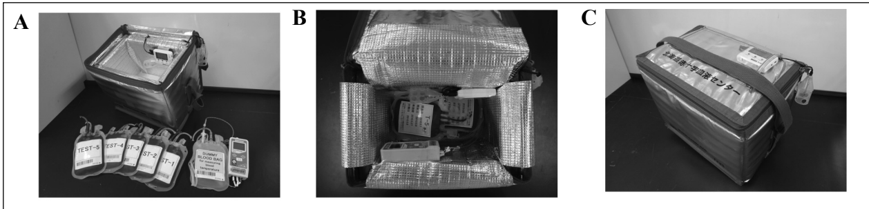
Figure 2 - A. The SS-BOX-110, equipped with an internal thermocouple probe to record the internal temperature and an outer probe to measure the ambient temperature during transport. The five units of red blood cell components and a dummy blood bag for recording the liquid temperature are also displayed. B. Five aliquots of red blood cells were put one by one in opposite directions after a bubble-sheet-wrapped frozen coolant had been placed on the bottom. Finally, the other wrapped frozen coolant was put on the top of the red blood cell bags, and a foam plug was used as the ceiling to ensure a tight fit. C. The container containing five bags of red blood cells, a dummy blood bag and two frozen coolants is shown. The outer thermocouple probe for measuring the ambient temperature and the data logger can be seen.
