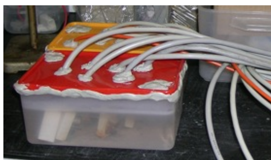
Figure 3. Photo of the PVC cell with the 12 sensors immersed in a thermostated solution.
