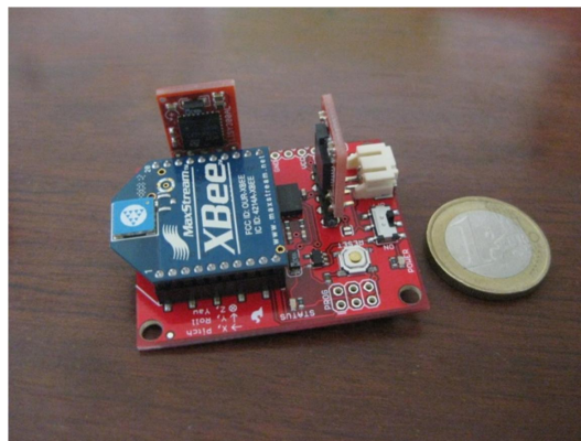
Figure 11. IMU used to validate the results.
