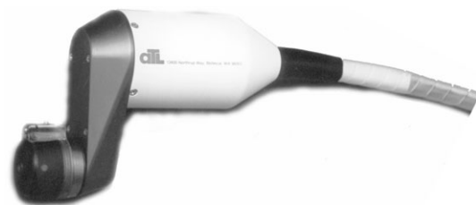
Figure 3. Early mechanically scanned transducer with the motor in the handle and three belt-driven transducers on the wheel.
