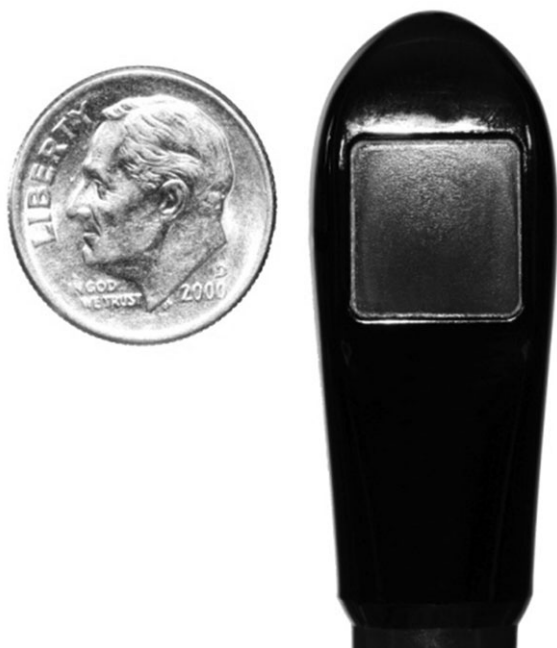
Figure 13. Philips X7-2 matrix transducer for imaging the heart in three dimensions in real time from within the oesophagus.
