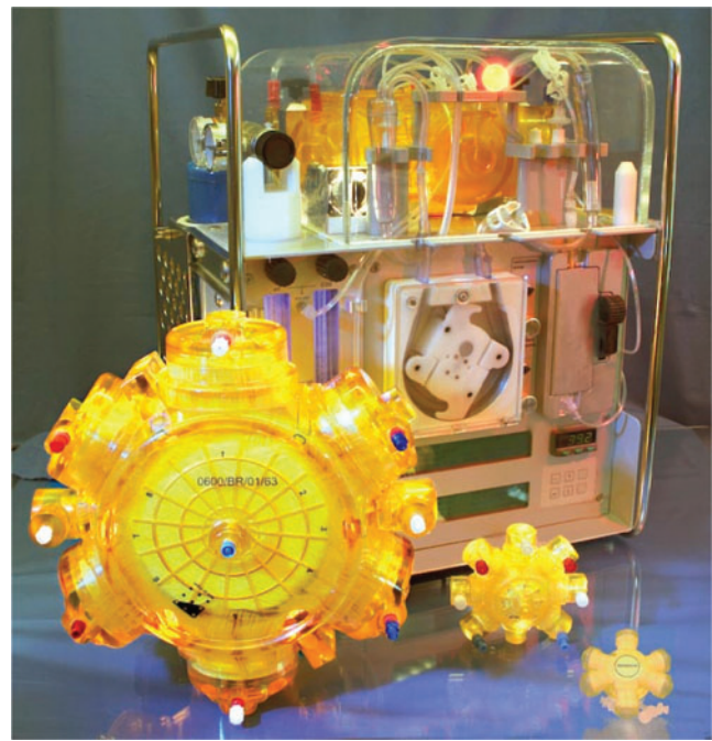
FIG. 2. Bioreactor and perfusion unit prototypes. Bioreactor perfusion system with pump heads for medium recirculation (left) and medium substitution (right); a heating chamber for bioreactor maintenance; rotameters for air, oxygen, CO 2 , and total gas flow; and a display for digital monitoring and regulation of perfusion parameters. Bioreactor prototypes with different cell compartment volumes (from the left to the right: 800, 8 and 2 mL) are shown in the front. Color images available online at www.liebertonline.com/tec
