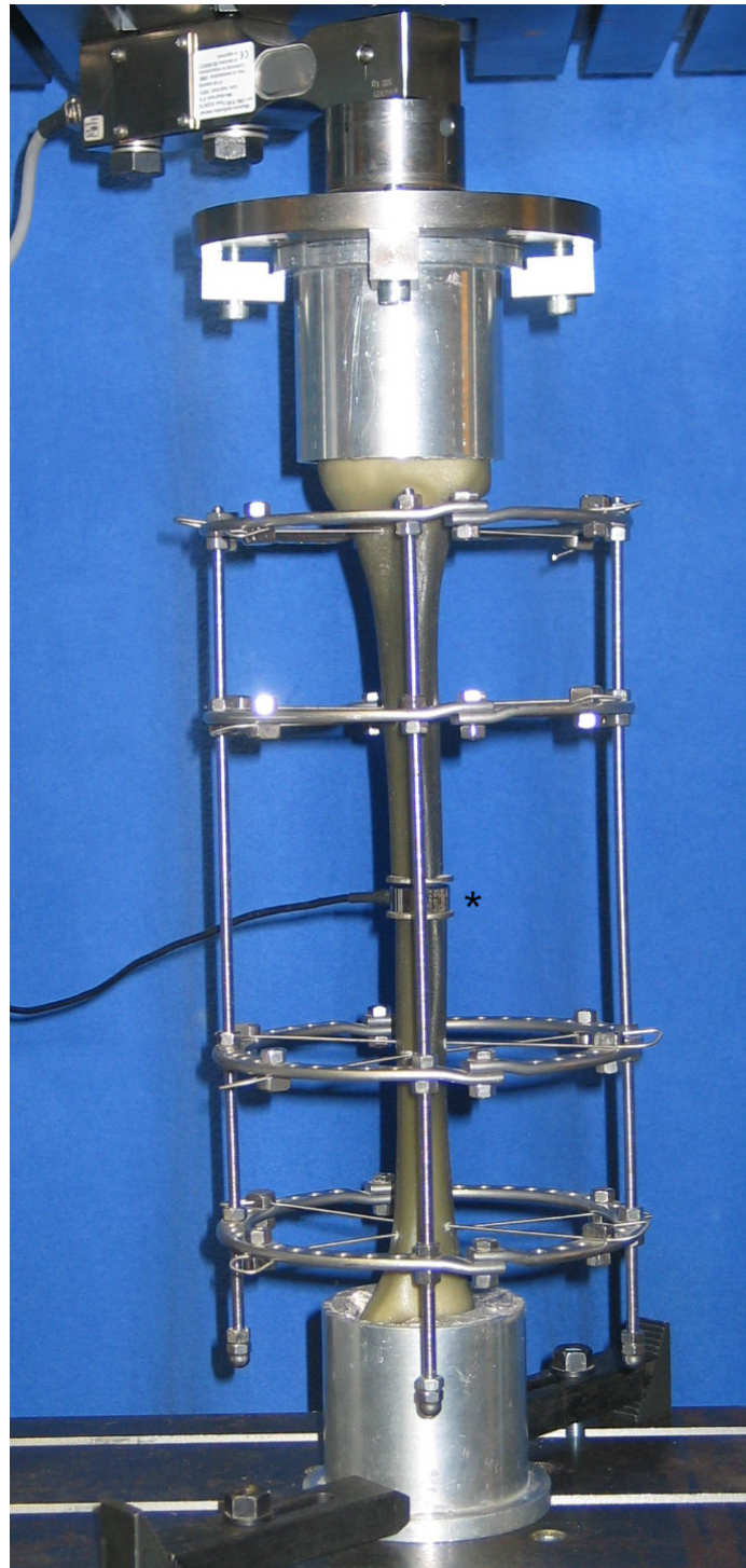
Figure 2 Experimental set-up of the wire frame under direct loading (both bone ends are mounted to the test machine) for measurements of the compressive loads in the osteotomy; the loading cell is placed into the osteotomy gap. (*) marks the loading cell in the osteotomy gap.
