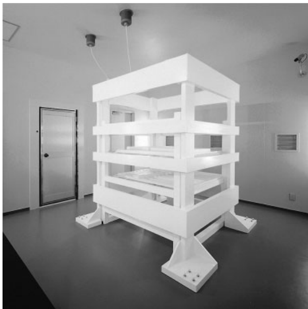
Fig. 1. Intermediate frequency (20 or 60 kHz) magnetic field exposure system for small laboratory animals. Two exposure systems were built; one for 20 kHz and another for 60 kHz. Their appearances and dimensions were identical so that the systems were interchangeable for the sham-exposure (control) system. Coil wires for 20 or 60 kHz MF were installed in four horizontal wooden bobbins of the respective exposure system. Distances between the four coils were 60, 41, and 60 cm. The sides of the square coils were 150 cm, and the height of the top coil bobbin from the floor was 222 cm. The Merritt-type four-square coils could produce uniform ( \pm 3\% ) 20 kHz MF up to 0.200 mT(rms) or 60 kHz MF up to 0.100 mT(rms) magnetic fields in a cubic space ( 100 \times 100 \times 100 cm) at the center of the coils where three wooden racks were layered to accommodate up to 36 rat cages in total. The magnetic field was vertical in orientation and sinusoidal in waveform.
