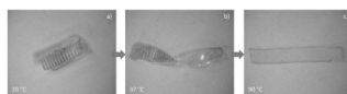
Figure 9. Sequential photographs taken of the recovery of a sample containing 10% UPyMA demonstrating the triple-shape memory effect. Recovery proceeded from the first temporary shape (bent and textured) (a) to the second temporary shape (twisted and textured) (b) and to the permanent shape (flat and smooth) (c).
