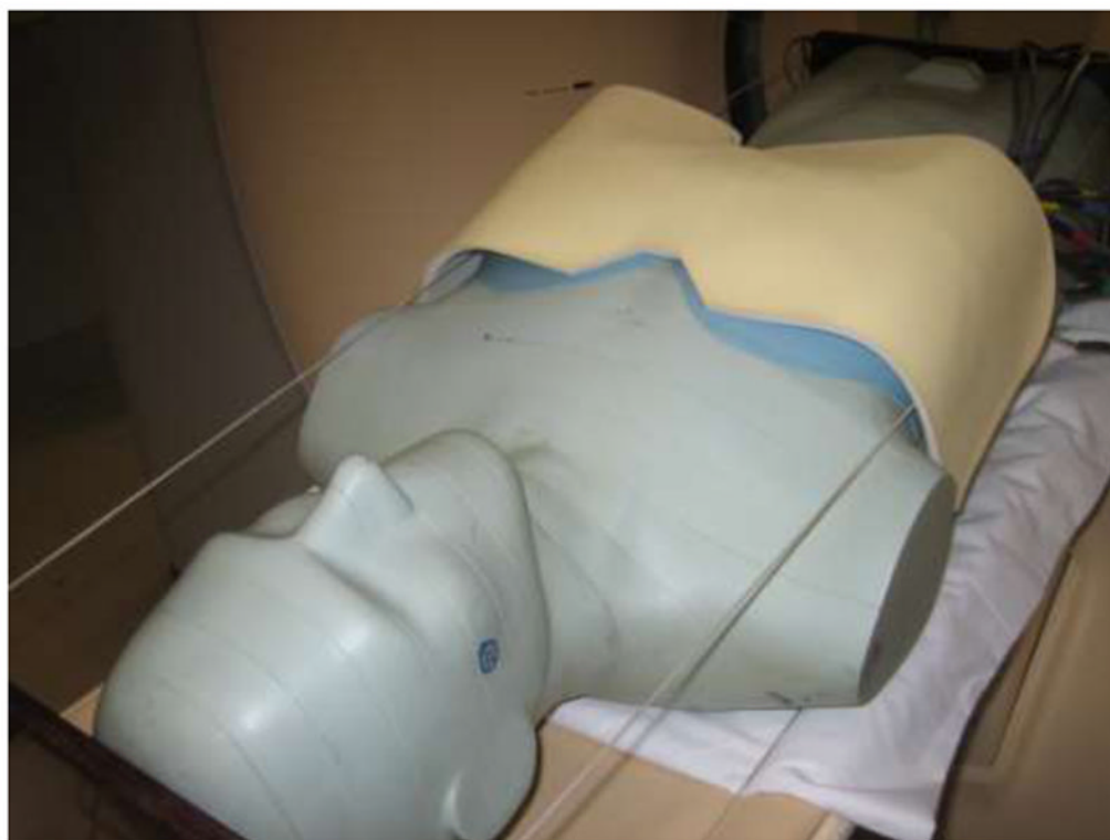
Figure 3. Phantom positioned on a scanner with bismuth breast shield in place. MOSFET detectors can be observed emerging from below shield in the upper right hand corner.
