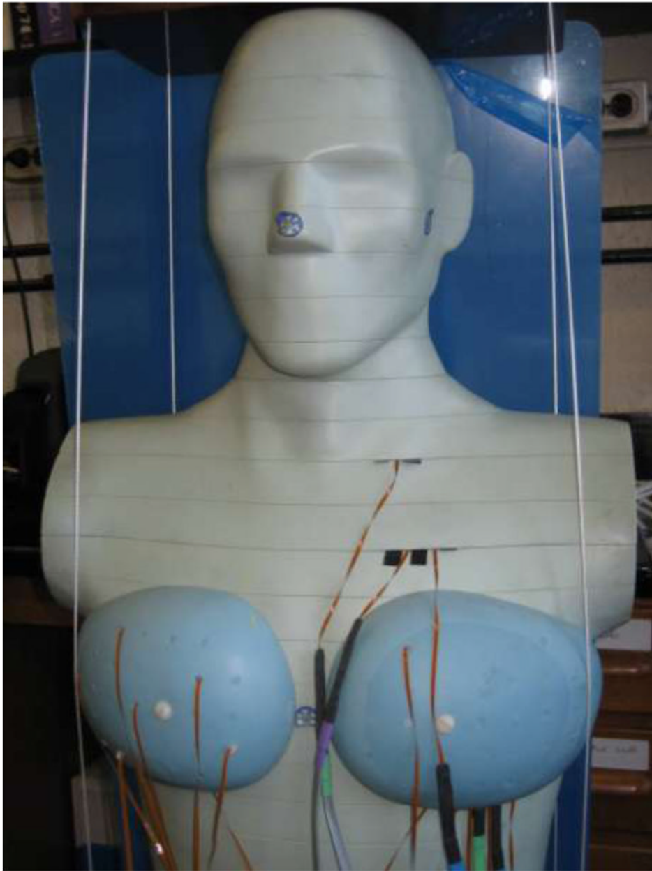
Figure 2. Phantom with MOSFETs attached to measure radiation doses to internal organs during CCTA. Here, MOSFETs are positioned both in breasts and internal organs for illustrative purposes.
