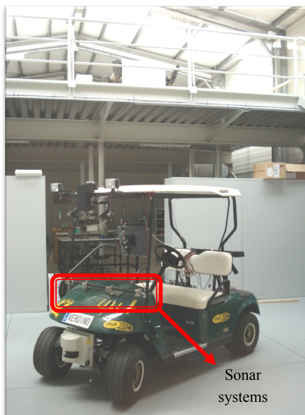
Figure 9. Photograph of the storework, the vehicle and the sonar systems.
