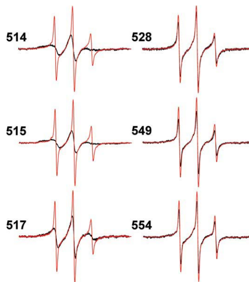
Figure 5. Effects of denaturant on EPR spectra of spin-labeled Tar. Normalized spectra for Tar in native membranes with spin labels at the indicated positions are shown in the absence (black) and presence (red) of 5M urea. Spectra were corrected for spin labels on other membrane proteins by subtracting the spectrum of native membrane vesicles containing Tar devoid of cysteine and treated with the spin-label reagent in the same way as vesicles containing the respective cysteine-containing form of Tar, scaled to total protein.
