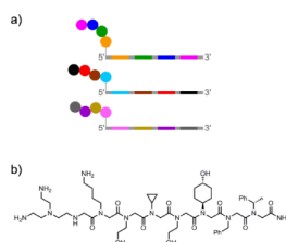
Figure 24. DNA display, in which distinct DNA sequences are used to route compounds through the combinatorial synthesis process. [110] a) Schematic depiction of three 'translated' small-molecule/DNA conjugates made using four DNA 'codons'. Not depicted is the split-and-pool approach used for each assembly step. b) An 8-mer peptoid ligand with K_d = 16 \mu\text{M} identified by DNA display. [111]
