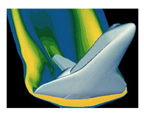
This Computational Fluid Dynamics (CFD) computer-generated image shows a model of the space shuttle. CFD has taken the place of wind tunnels for many evaluations of aircraft and, as computing power increases and computer models become more sophisticated, CFD will largely replace wind tunnels. Image credit: NASA.
