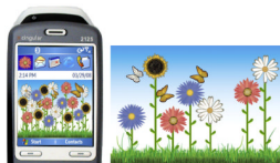
Figure 1. UbiFit's glanceable display on the phone's background screen. Different types of flowers represent different types of physical activities that the user performed this week (walking, cardio, strength training, and stretching). The butterflies indicate if the weekly activity goal was met this week (the large butterfly) and during the previous three weeks.
