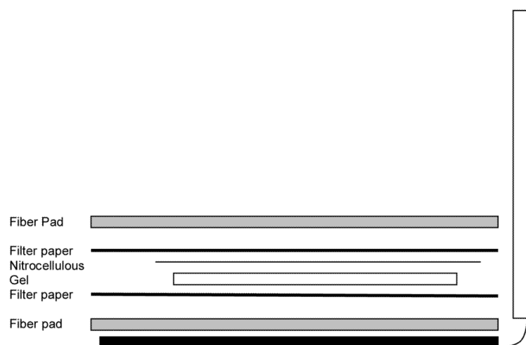
Figure 1. Schematic of immunoblotting preparation showing location of fiber pad, Whatmann paper, nitrocellulose and gel.
