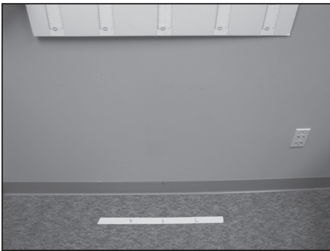
Figure 1. Each subject stood on an adhesive tape marker located on the floor parallel to and centered 15 cm from a wall containing a specially formulated board.
