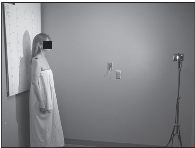
Figure 4. A high intensity light was utilized to cast a shadow of the retroreflective markers on the board. The light was centered on the board and was always positioned at the same height and the same distance from the board for all subjects.
