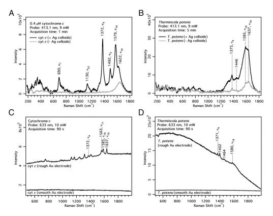
Fig. 3. Resonance Raman, SERS and SERRS spectra of cytochrome *c* and *T. potens* with 413.1 nm laser excitation (*A* and *B*) and 633-nm laser excitation (*C* and *D*) (*A*) 0.4  $\mu$ M cytochrome *c* and (*B*) *T. potens* in the presence (black traces) and absence (gray traces) of Ag colloids. (*C*) Cytochrome *c* and (*D*) *T. potens* on smooth and electrochemically roughened Au electrodes.
