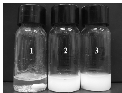
Figure 8 Pyrene (2.47 mM) in water (1) and with R3 (2, 100 \mu\text{M} ), or R4 (3, 100 \mu\text{M} ) in aqueous solution after stirring for 24 hours.
