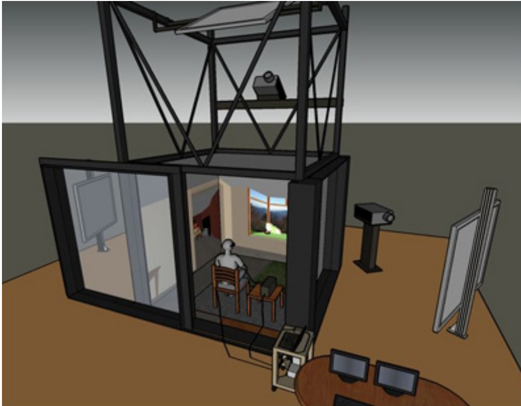
Figure 1. Schematic of the control room (VisRoom) and the DiVE cube with a human participant viewing a virtual scene.
