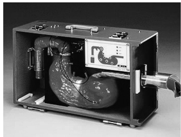
Fig. 1. The EGD simulator (Model LM022, Koken Co., Ltd., Toshima-ku, Tokyo, Japan). It consists of one opening for insertion on a box weighing 6.9 kg and measuring 51.8×28.8×18.8 cm. EGD, esophagogastroduodenoscopy.
