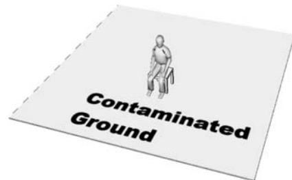
Figure 2. Ground contamination scenario showing a person in a sitting posture assuming isotropic planar source of ^{137}\text{Cs} (662 keV) under a 2-cm layer of soil with a concentration of 30 kBq m -2 .
