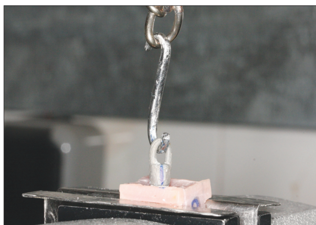
Figure 1: Luted metal coping during pull out test by universal testing machine
