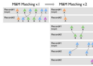
Figure 5. (left) M&M Matching v.1 (right) M&M Matching v.2 – Events in each event type are matched separately.
