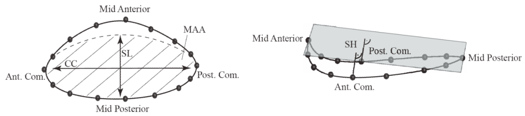
Fig. 2. Example of a piecewise cubic, three-dimensional spline, solid line, approximating the 16 marker coordinates in space, top view (left) and lateral view (right). We implant markers, black spheres, at the anterior and posterior trigones, at the mid anterior portion, at the mid posterior portion and at each commissure. Additionally, we place ten markers to subdivide the annulus into 16 segments of approximately equal length. The figure also illustrates mitral annular area (MAA), septal-lateral distance (SL), commissure-commissure distance (CC), and saddle height (SH).
