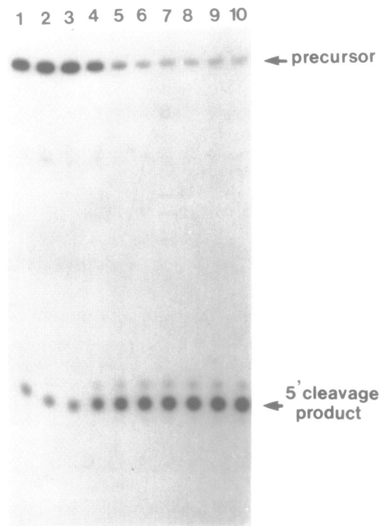
Figure 3. Self-cleavage of Rz89 at 37°C. The Rz89 precursor obtained by transcription at 4°C was 5' end-labeled with ( \gamma - 32 P)ATP and was further gel-purified. The radioactive Rz89 was denatured at 95°C for 1 min in 1 mM EDTA (lanes 1, 2, and 4 to 10) or 10 mM EDTA (lane 3) and snap-cooled on ice for 5 min. Tubes were then supplemented at 4°C with 40 mM Tris HCl pH 8.0 (lanes 2 and 3) or 40 mM Tris HCl pH 8.0 and 10 mM MgCl 2 (lanes 4 to 10), vortexed and spun down for 5 sec at room temperature, put again on ice and then incubated at 37°C. Aliquots were taken at time 0 (lane 4), 15 sec (lane 5), 30 sec (lane 6), 1 min (lane 7), 2 min (lane 8), 5 min (lane 9), 30 min (lanes 2 and 3) and 60 min (lane 10), and reactions were stopped by addition of 1 volume of 95% formamide/50 mM EDTA. In lane 1, the aliquot of ( 32 P)Rz89 was supplemented with formamide/EDTA gel loading buffer immediately after the snap-cool step. Samples were analyzed by PAGE 10%/7M urea as described in Mat. & Meth.
