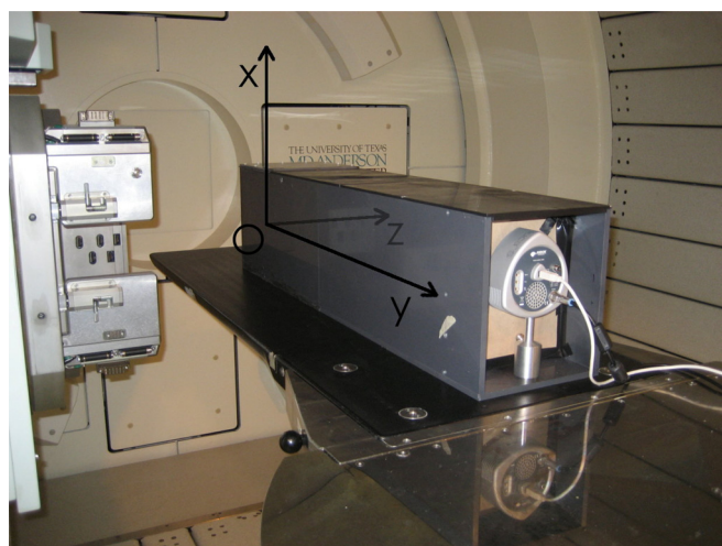
FIG. 1. The LS detector prototype with the coordinate system used throughout this work.
