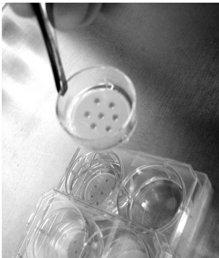
Figure 1. Photograph of the MRSA biofilms grown on tissue culture inserts. The insert (25 mm in diameter) is placed in a well of a 6-well plate.
