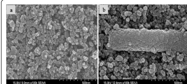
**Figure 2** FE-SEM images of (a)  $\text{TiO}_2$  film and (b) 5 wt.%  $\text{ZrO}_2$  nanofiber-doped  $\text{TiO}_2$  film.
