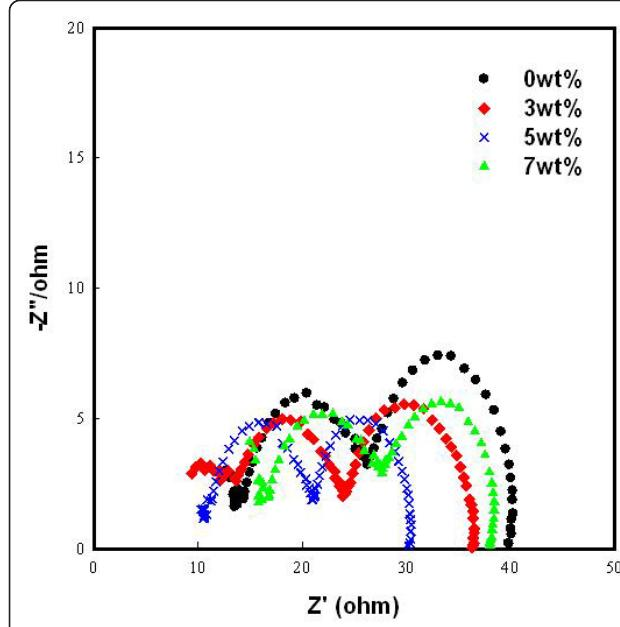
**Figure 5** Nyquist plots of the DSSCs using  $\text{TiO}_2$  film and  $\text{ZrO}_2$  nanofiber-doped  $\text{TiO}_2$  film. Black circle, 0 wt.%; red diamond, 3 wt.%; cross mark, 5 wt.%; green triangle, 7 wt.%.
