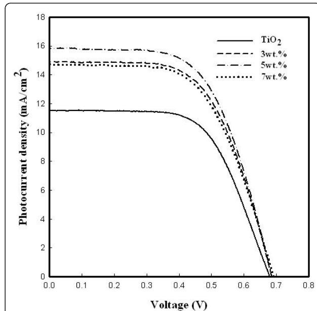
**Figure 6** Photocurrent-voltage curve of the  $\text{TiO}_2$  film and the  $\text{TiO}_2$  films with  $\text{ZrO}_2$  nanofibers.
