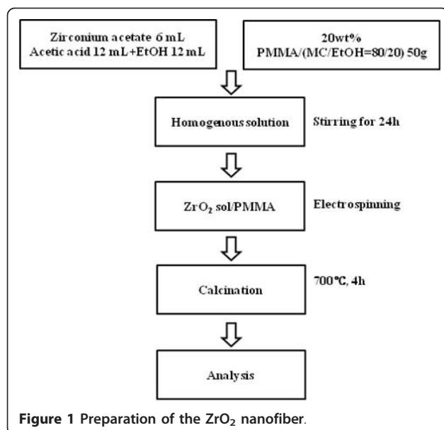
**Figure 1** Preparation of the  $\text{ZrO}_2$  nanofiber.
