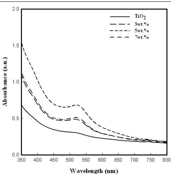
**Figure 4** UV-Vis spectrum of  $\text{TiO}_2$  film and  $\text{ZrO}_2$  nanofiber-doped  $\text{TiO}_2$  film after 24-h dye absorption.
