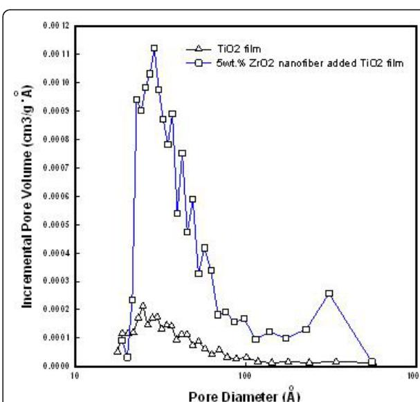
**Figure 3** BJH curve of  $\text{TiO}_2$  film (triangle) and 5 wt.%  $\text{ZrO}_2$  nanofiber-doped  $\text{TiO}_2$  film.
