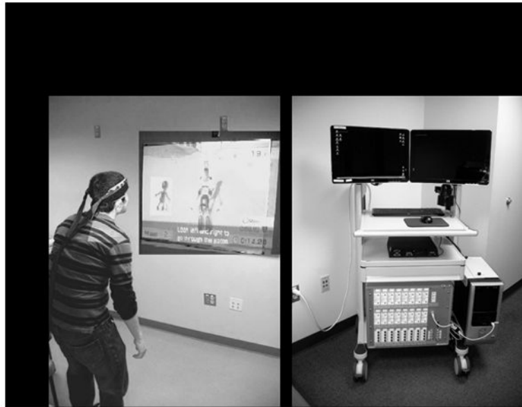
Figure 2. FNIRS signals were recorded from subjects during upright performance of the balance task (panel A). A 32-channel fNIRS system (shown in panel B) was used to collect the data. Ten (10) meter long fiber optics were used to transmit and receive the signal from the bilateral head cap worn by the participant and the fNIRS instrument.
