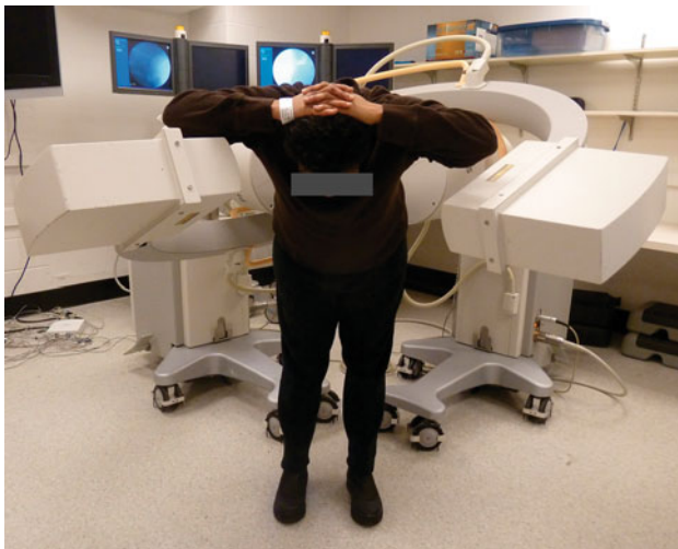
Fig. 1 Experimental setup of the dual-fluoroscopic system (DFIS) for capture of the lumbar spine positions in vivo
