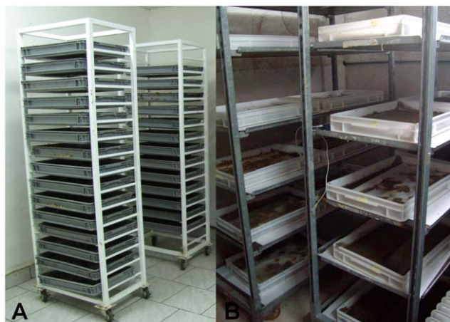
Figure 2. Trolleys with larval trays for biodegradation. (A) Miloslavov trolleys (maximum capacity 75 kg of manure) and (B) Alpuente trolleys (maximum capacity 64 kg of manure). doi:10.1371/journal.pone.0032798.g002
