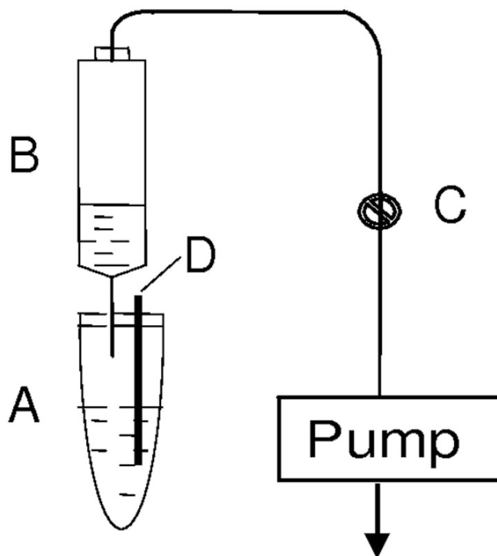
**Fig. 2.** Schematic illustration of the aldehyde-generating and trapping apparatus. A: Microsomal incubation mixture; B: LpDNP cartridge; C: Two-way valve; D: Hypodermic needle (for aspiration of the system and agitation of the mixture).
