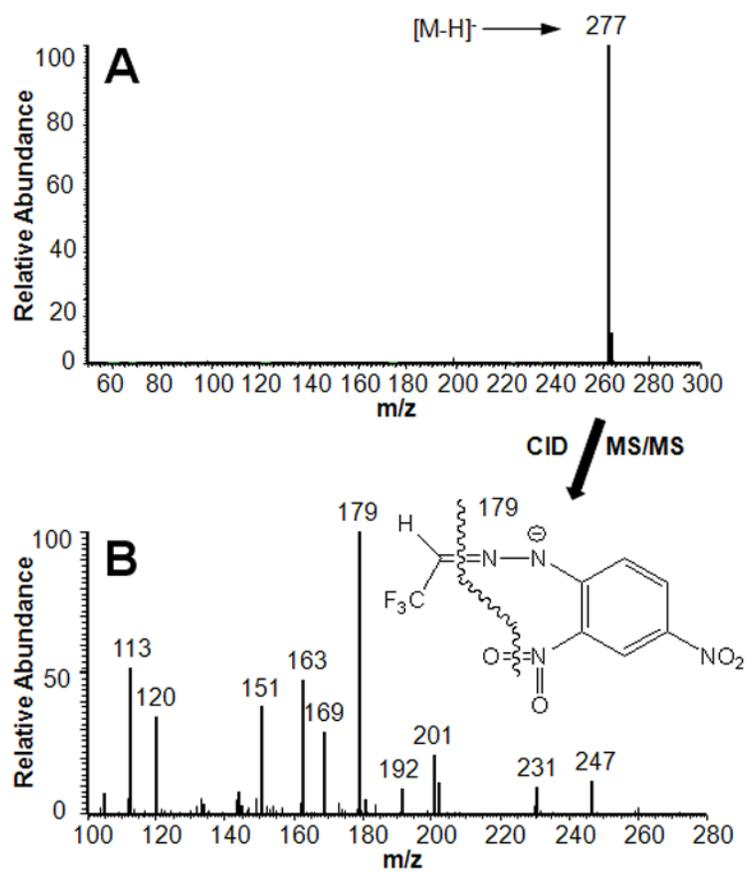
**Fig. 6.** Full-scan LC-ESI-MS of TFAA-DNPH (A) and CID-MS/MS spectrum of the  $[M-H]^-$  ion,  $m/z$  277 (B).
