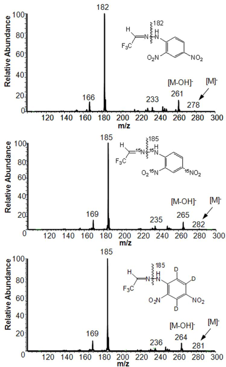
Fig. 5. Full-scan GC-NCI-MS of TFAA-DNP and its  $^{15}\text{N}_4$ - and  $\text{d}_3$ -labeled analogues.
