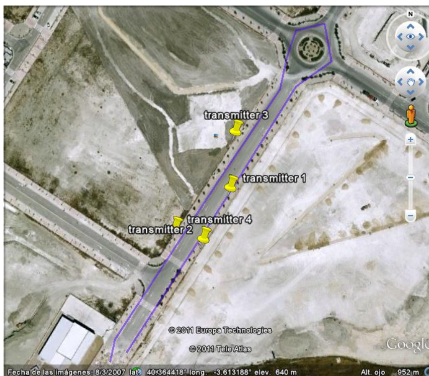
Figure 15. Test-bed. In violet color, the path of the car. In yellow, the four transmitters.
