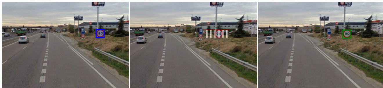
Figure 10. (Left) Left image and bounding box of the detected speed sign; (Middle) Search space along the epipolar line corresponding to the upper-left part of the bounding box on right image; (Right) Final match on right image.
