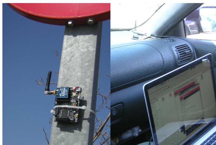
Figure 13. (Left) Wasp mote transmitter installed on a signal. (Right) Wasp mote receiver in the test-car.
