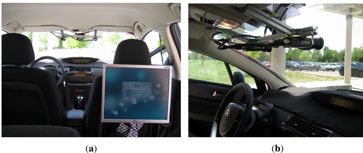
Figure 1. (a) Inside view of the experimental vehicle (a modified Citroën C4); (b) Stereo vision sensor.
