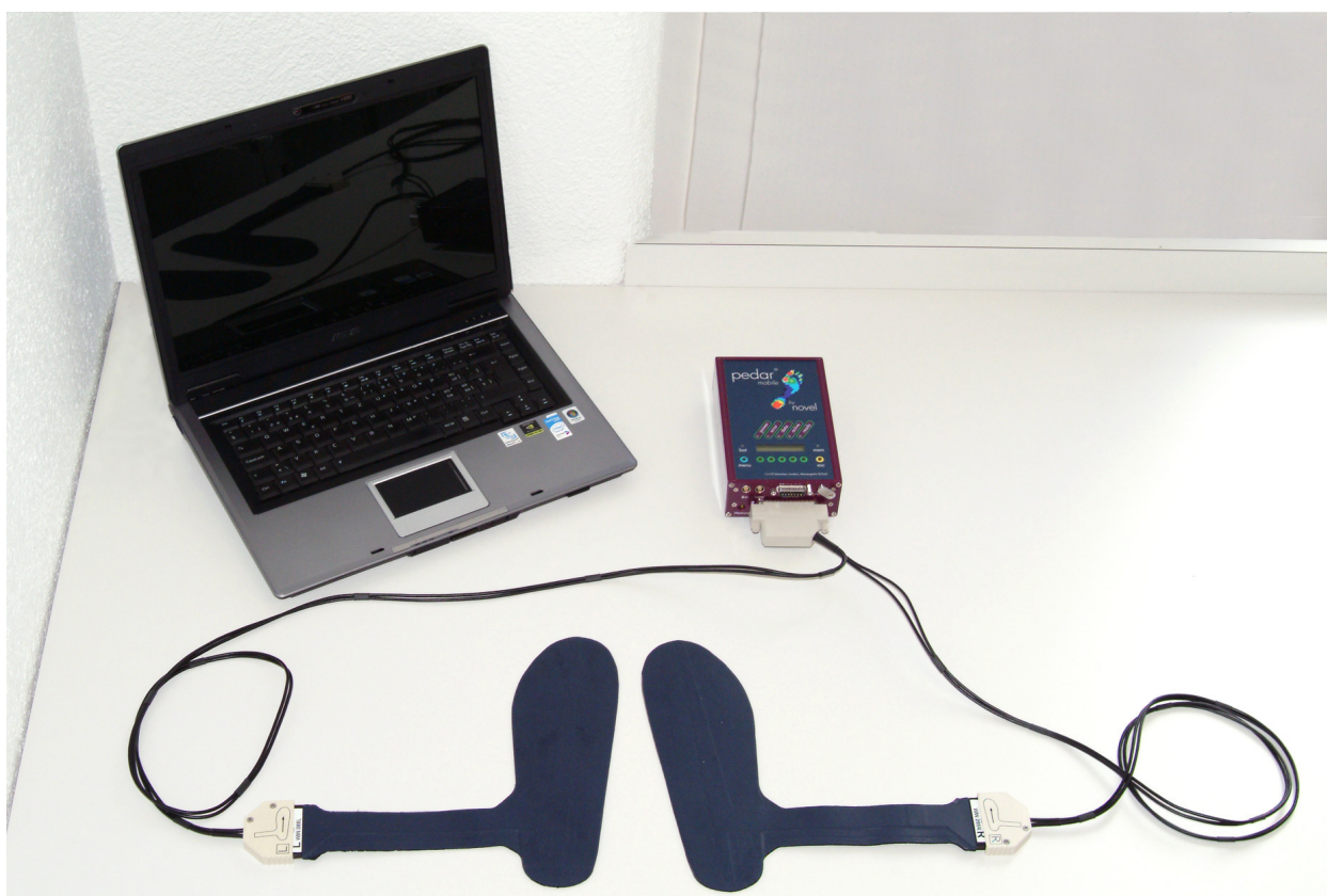
Figure 2 Pedar mobile system. Illustration of the Pedar Mobile system with the matrix insoles that are connected to the recording device. This device is further connected to a personal computer with the respective software to evaluate the measurements.
