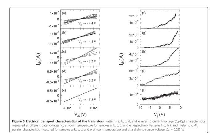
keeping a fixed  $V_{\rm sd} = 0.025$  V value. In all cases, at negative gate voltages, the electric field is able to produce a depletion region narrowing the channel and turning off the current flowing through the nanowire when  $V_g$  approaches the pinch-off voltage value. In the last case (Figure 3 patterns e and l), the gate potential is indeed not able to remove the electrons and a current still flows through the channel even at  $V_g = -10$  V.
