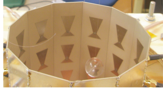
FIGURE 22: Second cavity with antennas designed to operate at 915 MHz of Experiment 2. Three acrylic sphere are suspended (one visible). Cavity is filled with fluid for imaging.
