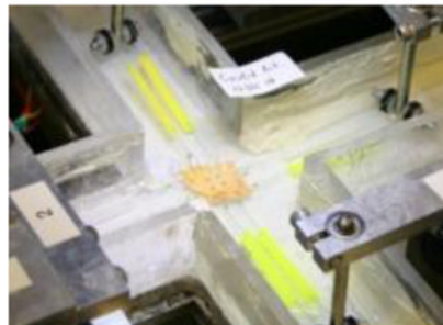
(b) Tissue sample mounted for biaxial test.
