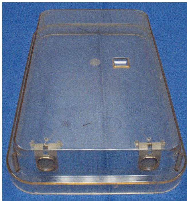
Figure 3. Top view of cage lid for the ndIVC, showing the absence of any filter and the 2 spring-loaded, flap ports through which incoming and outgoing air exchange occurs once the IVC is mounted on the ventilation rack.
