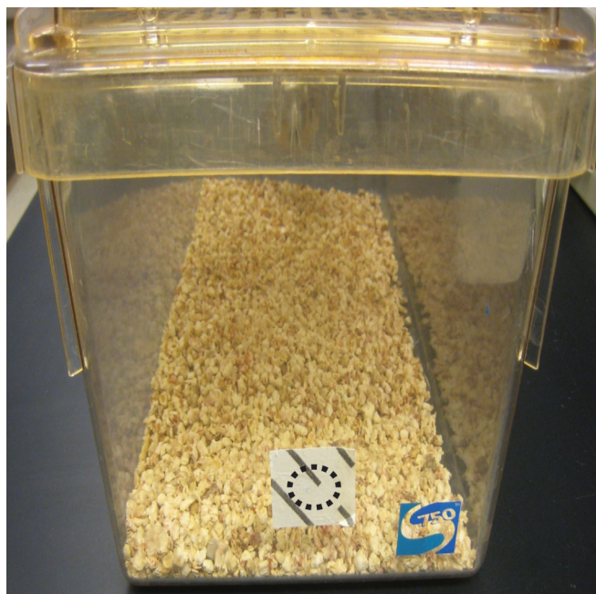
Figure 1. Cage modification. A 1/4-in.-diameter hole was drilled in the front of a microisolation mouse cage, 4 cm from the cage bottom. Dotted line indicates location of hole in cage wall.
