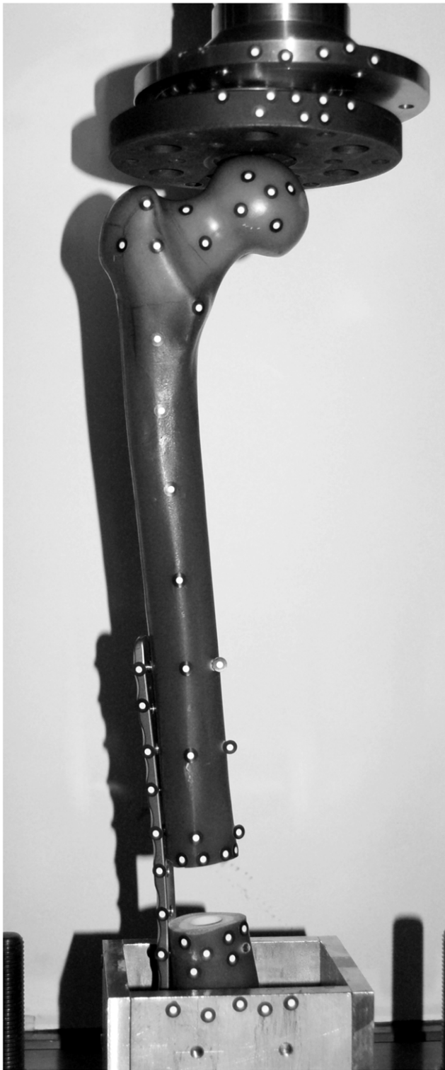
Figure 5. Experimental test setup. Posterior view of the test arrangement with a composite left femur mounted in the universal testing machine (Zwick/Roell). Segmental defect is bridged with an osteosynthesis system on the lateral (outer) side and fixed with seven titanium screws. Distal end of the femur is embedded in a metallic socket, filled with casting resin. 57 optical markers were attached onto the femur, socket and the testing machine to calculate their displacement during loading. doi:10.1371/journal.pone.0033776.g005
