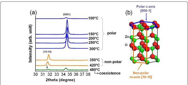
**Figure 1 XRD results.** (a) XRD plots for ZnO films grown at substrate temperature from 100°C to 480°C. (b) The wurtzite ZnO structure model with the illustrations of (0001) and (10-10) planes, corresponding to the structure shown in (a).
