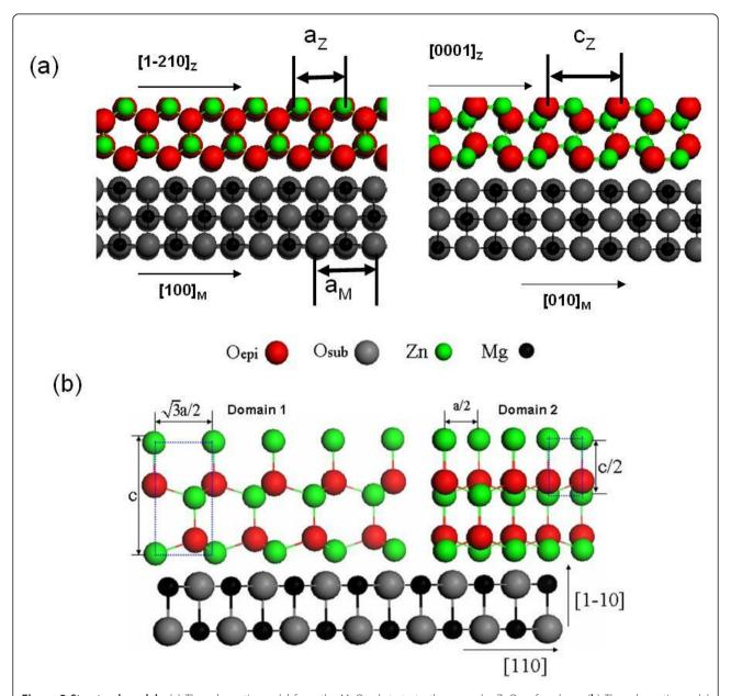
**Figure 3 Structural models.** (a) The schematic model from the MgO substrate to the nonpolar ZnO surface layer. (b) The schematic model from the MgO substrate to the polar ZnO surface layer.
