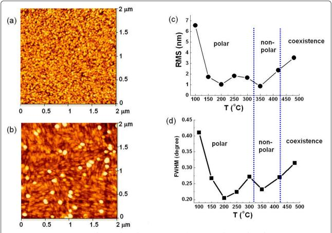
**Figure 4 AFM results**. (a) AFM image of the ZnO film surface grown at 150°C. (b) AFM image of the ZnO film surface grown at 420°C. (c) The evolution of surface roughness as a function of substrate temperature. (d) The evolution of XRD FWHM values as a function of substrate temperature.
