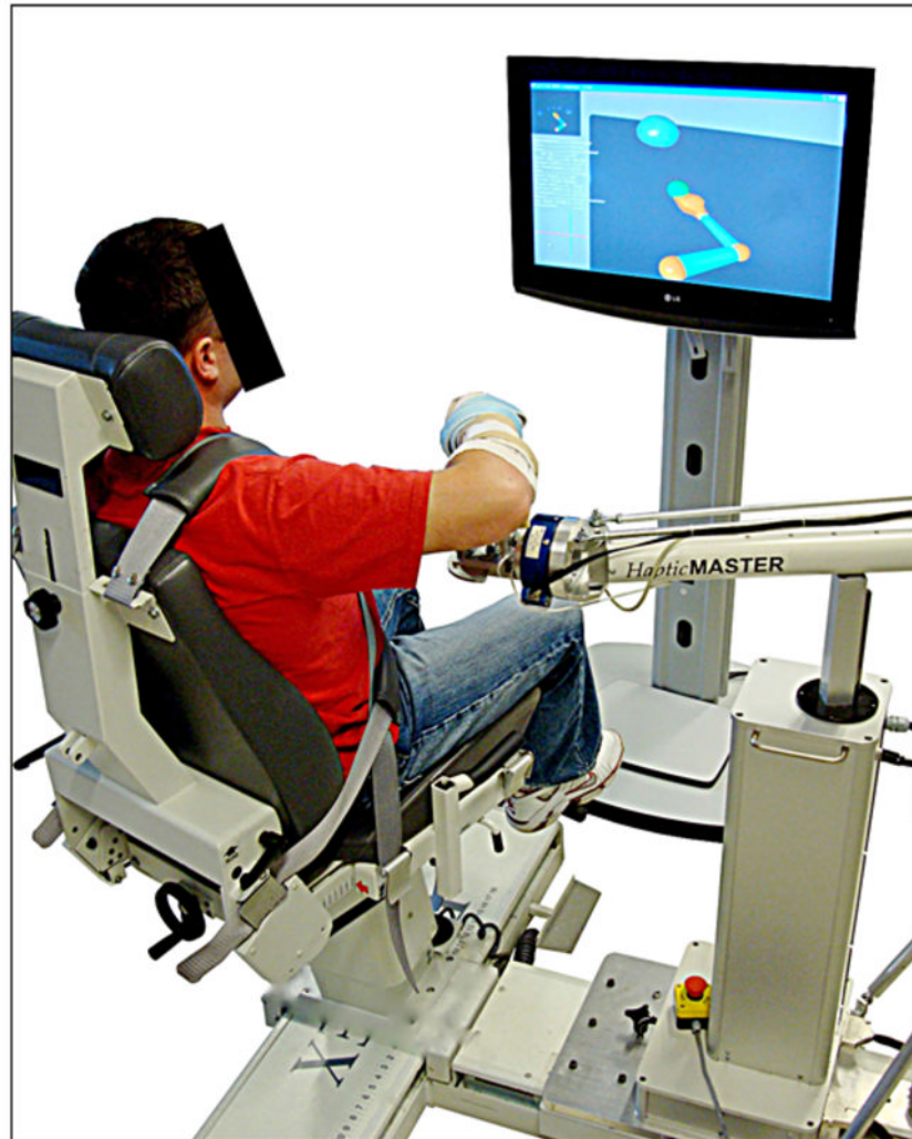
Figure 1. Experimental setup. Arm Coordination Training 3D system* provided haptic interface to simulate various loading conditions while subjects performed arm reaching movements with avatar and game feedback. *Sukal TM, Ellis MD, Dewald JP. Shoulder abduction-induced reductions in reaching work area following hemiparetic stroke: Neuroscientific implications. Exp Brain Res. 2007;183(2):215–23.[PMID: 17634933] DOI:10.1007/s00221-007-1029-6
