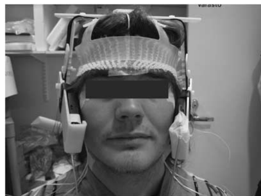
Figure 2 Frontal view of a subject and the exposure setup. Two modified phones attached to a plastic helmet were placed against each ear, mimicking the natural position during mobile phone use. Five temperature probes were attached to the head skin with adhesive tape, and three of them are shown here on the forehead and at both outer eye corners.
