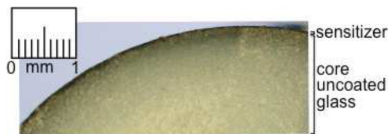
Figure 3. A low-magnification (10 \times ) cross-sectional optical image. The dark green thin coating shows the depth of 1 accessed into PVG. The image shows \sim 0.08 mm penetration depth on the outer face of the cylinder-shaped PVG cap 1 (diameter 5.0 mm \times length 8.0 mm).
